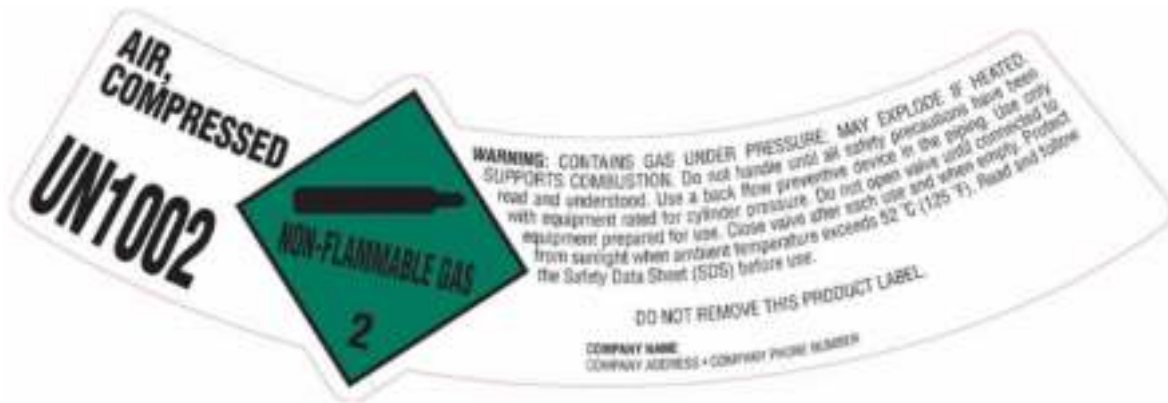
Figure 4: Example of an Air, Compressed cylinder shoulder label
