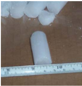
Extruded dry ice pellets (5/8 in [1.588cm])
