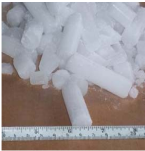
Extruded dry ice pellets (5/8 in [1.588cm])
