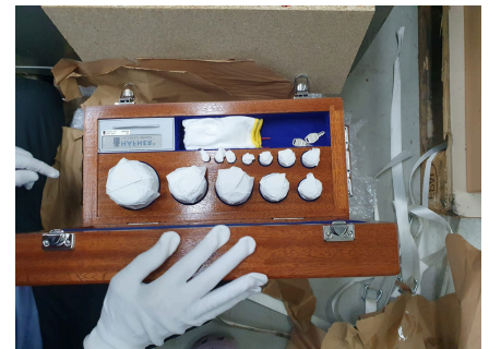
Set of E1 from 1 mg to 20 kg including handling instrumentation
